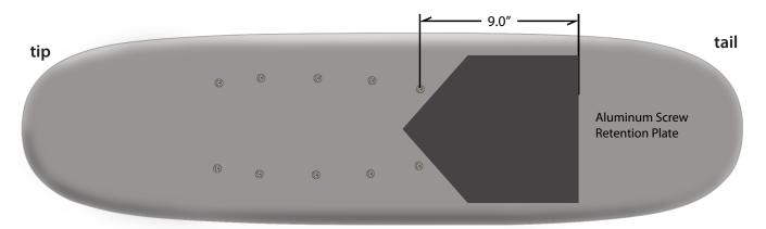
All AIRA trick skis have front boot machine screw inserts for mounting. Do not drill into areas of the ski other than where the aluminum retention plate is located. We suggest using our D3 Pro Trick Plate (PTP) for maximum adjustment and to prevent heel dents.
